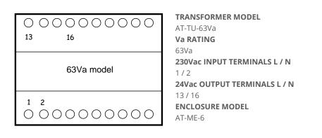
The transformer has a PTC circuit and overload protection for the voltage input. If the unit trips on the PTC overload - turn off the input Voltage for 1 or 2 minutes to manually reset the transformer. Reset will not occur automatically. This is a safety feature of this transformer.
